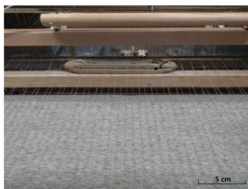
Fig. 1. Picture of the weaving operation of the QUDH fabric on a Leclerc Weavebird loom
